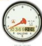
Read the mechanical odometer numbers from left to right. The meter shown in the image reads 369,200 gallons.
