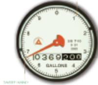
Observe that the water meter has one dial with a sweep hand and scale numbered from 1 to 10. Each revolution of the sweep hand represents 10 gallons of water through the meter.
